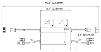
Our flagship product, the APS YC500A is a grid-tied microinverter with intelligent networking and monitoring systems to ensure maximum efficiency. Highly dependable and cost effective, the YC500A handles up to 310W modules with negligible clipping, delivering 250W AC per module with dual MPPT. Half the inverters and half the installation means real cost savings for residential and commercial customers.
